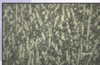
Interplate IP800 AS2576-2480 austenitic complex chromium carbide overlay x100mag
